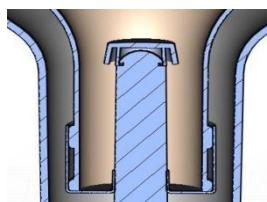
4. Valve automatically closes when bottle is removed. If bottle is not empty, water will not spill.
