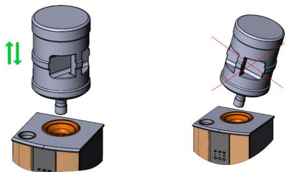
3. Opening finger automatically opens cap valve and keeps it open until bottle is removed.
